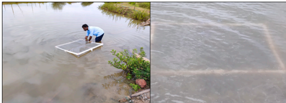
Fig. 6. Substrate-based bioreactor deployed at field.
