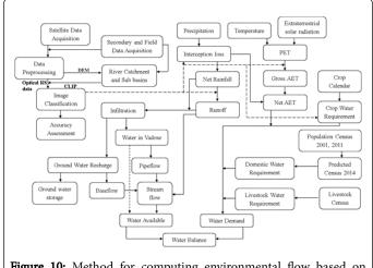
Figure 10: Method for computing environmental flow based on hydrologic variables.
