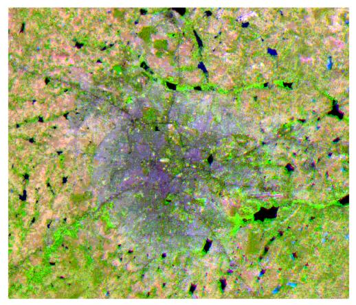
FIGURE 4: FCC OF BANGALORE CITY SHOWING RADIAL PATTERN OF GROWTH FROM THE CITY CENTRE AND LINEAR PATTERN ALONG THE HIGHWAYS
