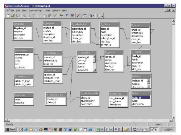
Figure 2: E-R Diagram of the entire database design
