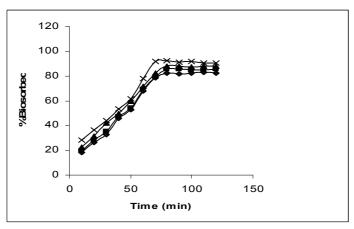
Figure. 3: Effect of contact time on the adsorption of fast green by coffee husk ( $\diamond$  10 mg/L 20 mg/L  $\blacktriangle$  50 mg/L x 100mg/L)
