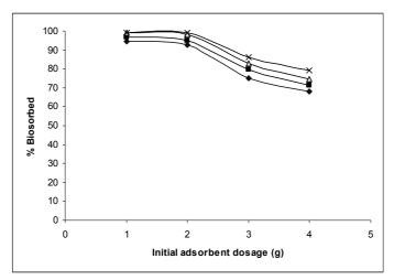
**Figure. 2:** Effect of adsorbent dosage on adsorption of fast green respectively by tamarind pod shells (♦ 10 mg/L ■20 mg/L ▲ 50 mg/L x 100mg/l)
