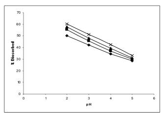
Figure. 1: Effect of pH on the fast green adsorption respectively by coffee husk( $\diamond$  10 mg/L  $\blacksquare$  20 mg/L  $\blacktriangle$  50 mg/L x 100mg/l)
