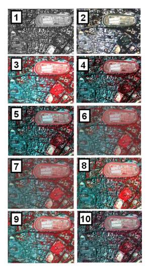
Figure 1. Original PAN image (1), original LR MS image (B-G-R) resampled at 1 m pixel size (2), original LR MS image (G-R-NIR) resampled at 1 m pixel size (3), Fusion through IHS (4), BT (5), HPF (6), HPM (7), PCA (8), FT (9) and CA (10).
