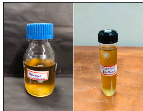
Fig. 13. Biodiesel extracted from the field harvested microalgal biomass.
