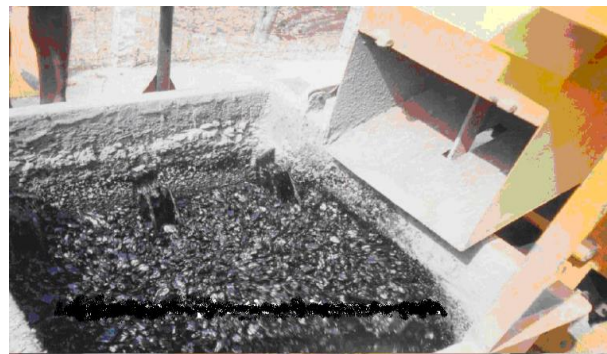
Aggregate-plastic- Bitumen Mix
