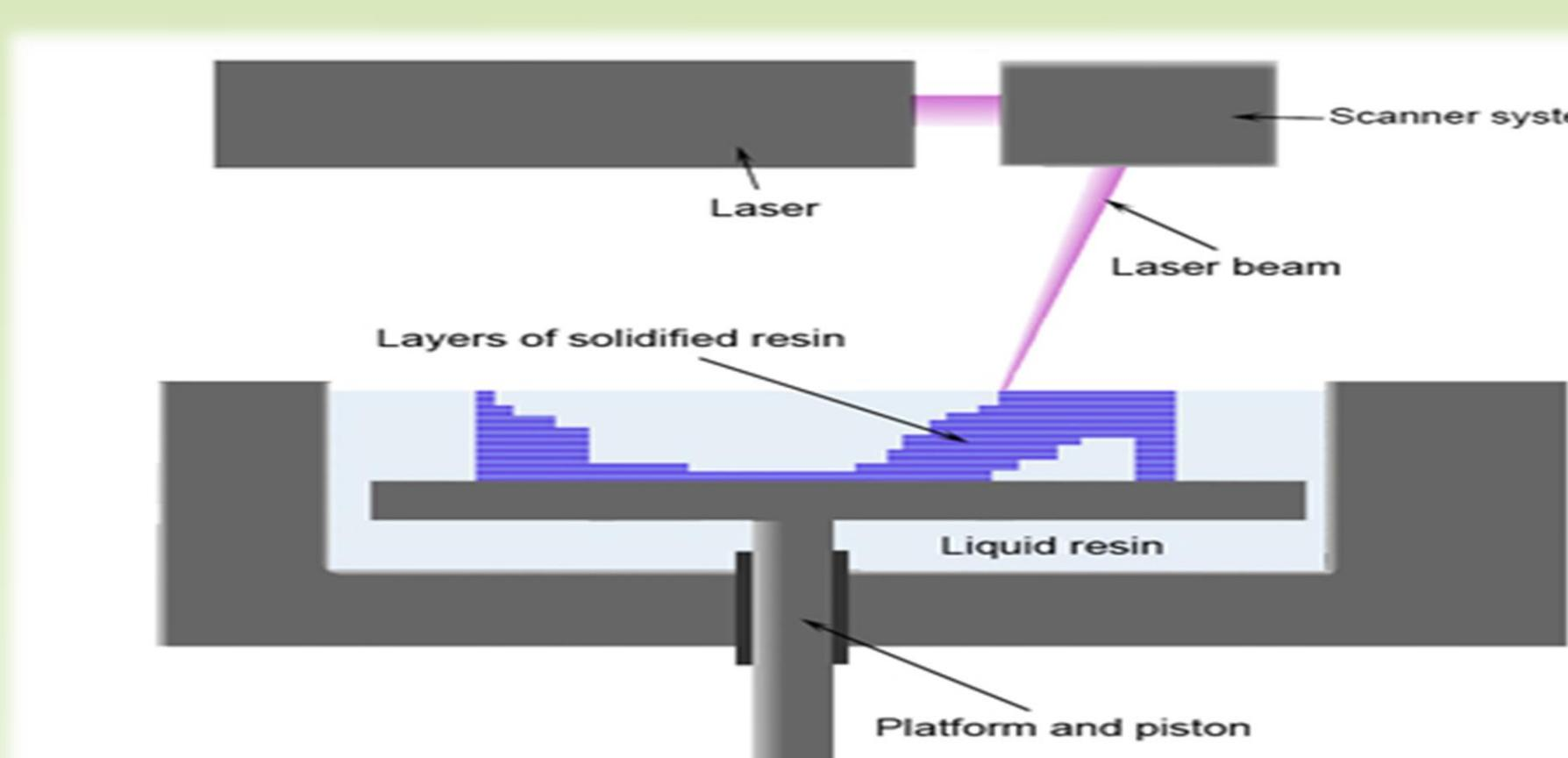
Stereolithography is an additive manufacturing process which employs a vat of liquid ultraviolet curable photopolymer "resin" and an ultraviolet laser to build parts' layers one at a time.
