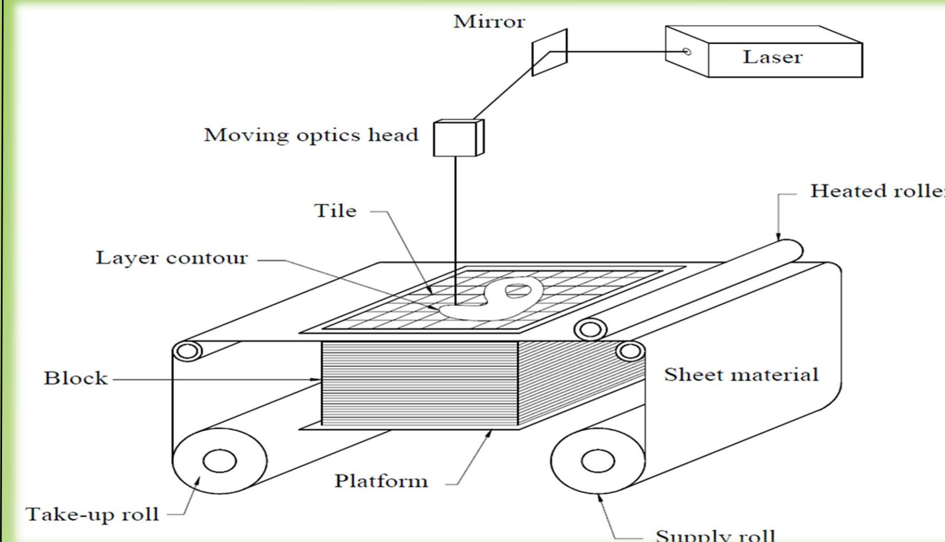
Laminated object manufacturing (LOM) is a rapid prototyping system developed by Helisys Inc. In it, layers of adhesive-coated paper, plastic, or metal laminates are successively glued together and cut to shape with a knife or laser cutter. Objects printed with this technique may be additionally modified by machining or drilling after printing. Typical layer resolution for this process is defined by the material feedstock and usually ranges in thickness from one to a few sheets of copy paper.
