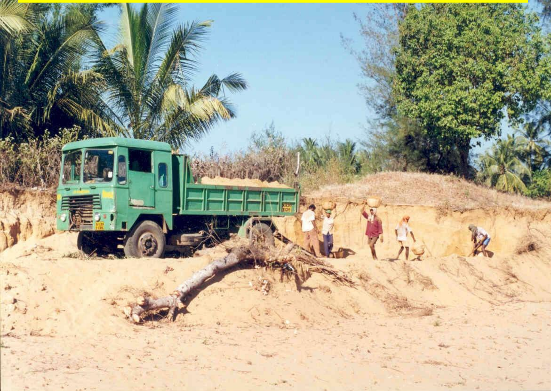
Dune sands- actively mined for construction purpose, north of Karwar town.
