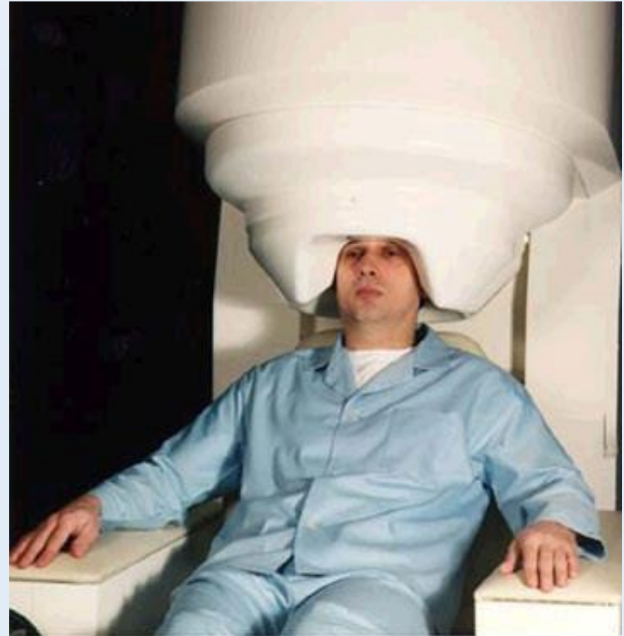
Multichannel whole cortex system with a concave bottom dewar (Illustration)
