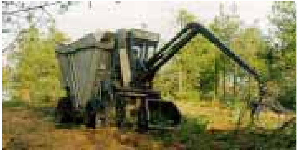
In Denmark, special equipment is used for collection and chipping of forest residues.
