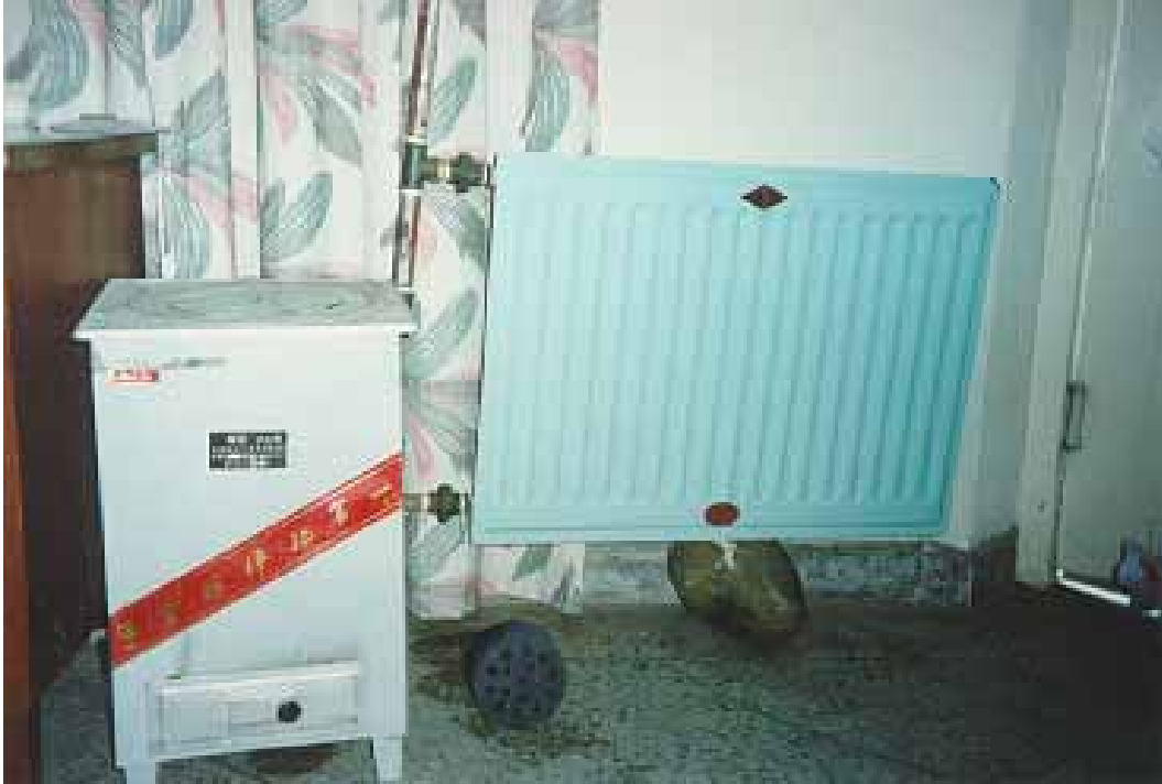
Above: Another view of the Chinese cooking and heating stove produced and sold commercially by the National Structure and Engineering Company, Nepal; Below right: One of the many types of metal cooking and heating stove sold commercially in Nepal.
