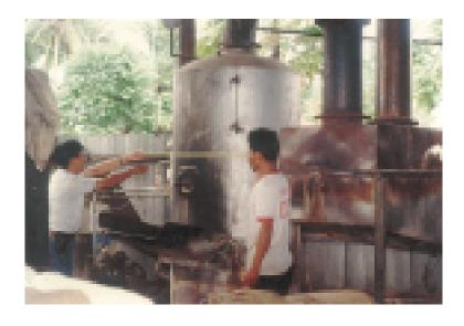
Biomass fired steam boiler used to provide process heat for noodle production (steaming)
