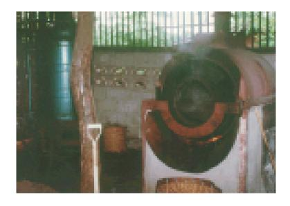
Wood fired boiler for generating the steam which is used for fermenting tea (miang)
