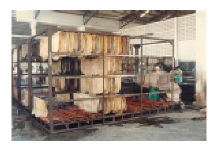
Rubber sheets hanging over supporting rods for smoking/drying in the kiln
