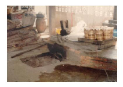
Wood fired furnace with steamer. Fish are packed in bamboo/rattan containers for steaming
