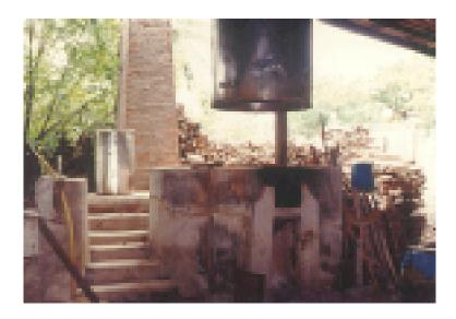
Wood fired furnace with vinegar distillation unit
