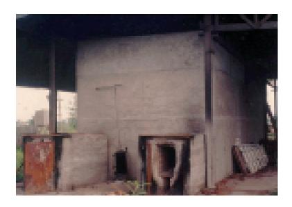
Wood fired drying chambers for drying the parquet
