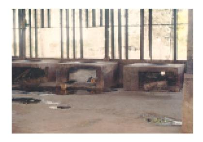
Wood fired furnaces with pots in which water is boiled for dehairing carcasses
