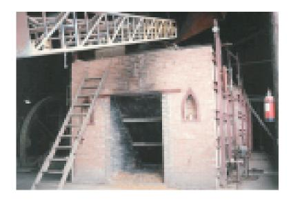
Rice husk fired furnace with step grate which provides process heat for generating the steam which is used to drive the equipment
