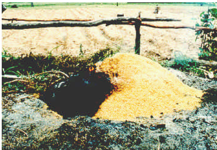
Charcoal Making in Shallow Pit Kiln, Covered with Rice Husk
