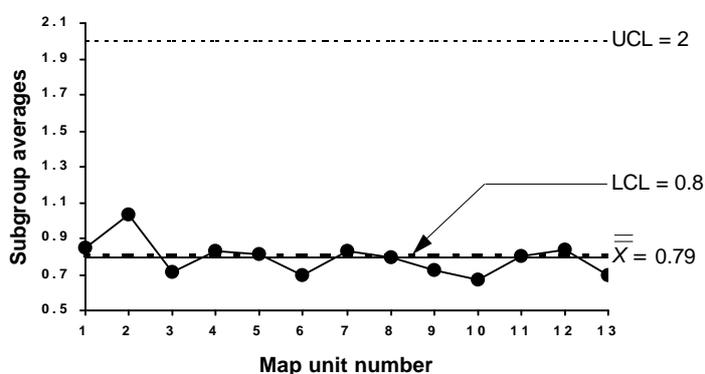
Figure 10.  $\bar{X}$  chart based on acceptance limits for soil OC.
