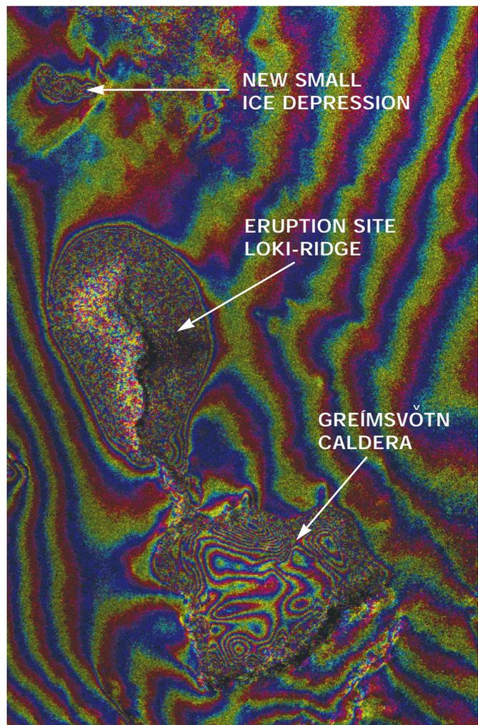
FIGURE 13 Interferogram from ERS-1 and ERS-2 images taken two days apart (Vatnajökull volcano, Iceland). The pear-shaped depression in the middle of the image is the volcanically active area (source: DLR, Germany)
