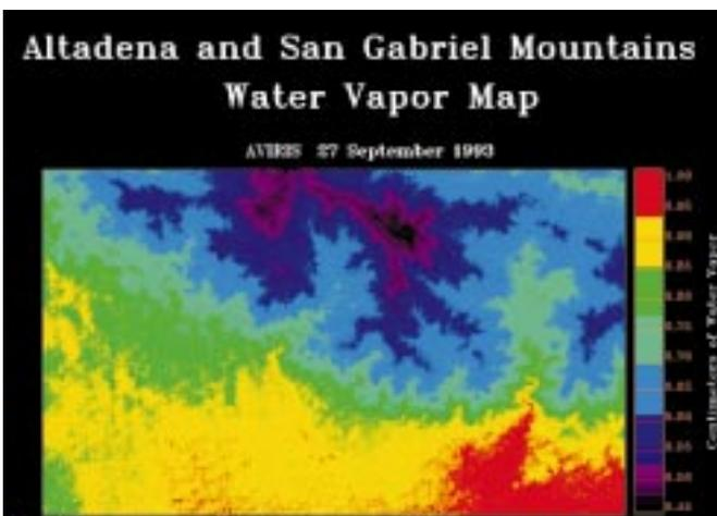
FIGURE 11 Water vapour map prepared using AVIRIS (source: NASA)
