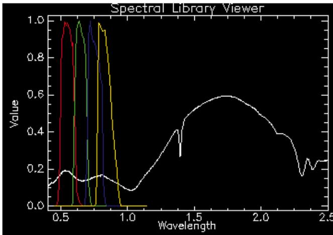
FIGURE 7 Spectral reflectance curve for mineral with Landsat MSS absorption bands superimposed in colour
