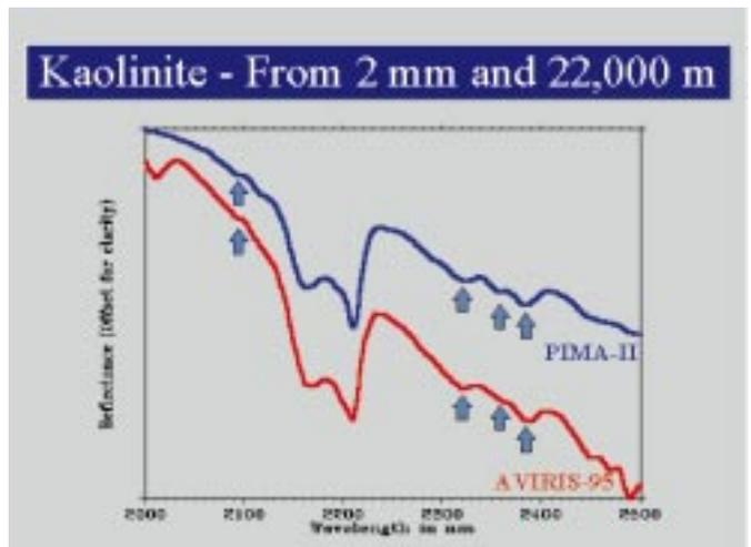
FIGURE 10 Reflectance of kaolinite from 2 mm (PIMA-II) and 22 km (AVIRIS) (source: NASA)
