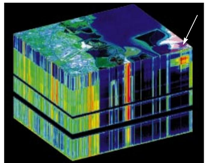
FIGURE 12 Image cube prepared using AVIRIS (source: NASA)
