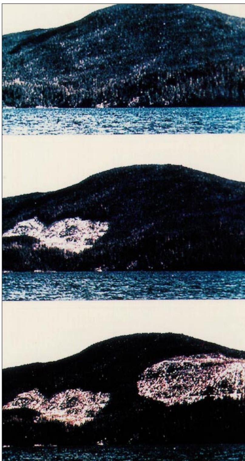
**FIGURE 18** Visualization of proposed forest operations. Aerial photographs draped on a DEM "wire frame"
