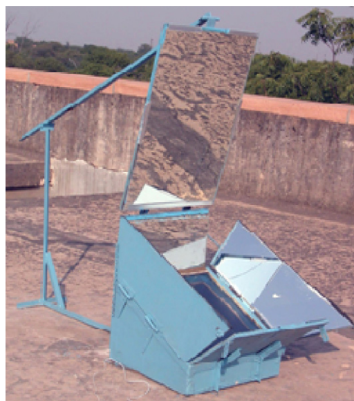
Fig. 5. Modified solar cooker with booster mirror [72].
