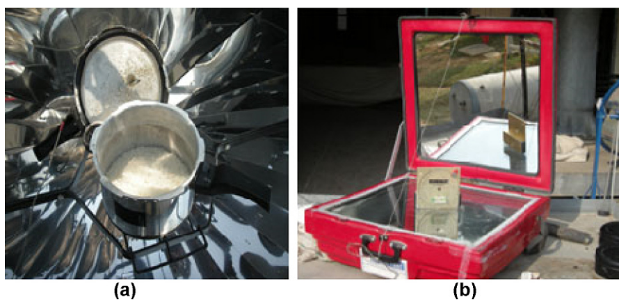
Fig. 9. (a) Paraboloid cooker with food stuff and (b) the photographic view of box-type solar cooker [87].
