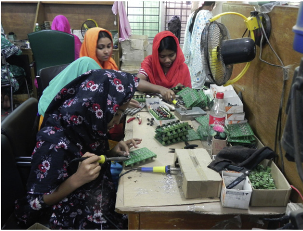
Fig. 3. Women assembling solar charge controllers at an electronic unit in Dhaka.
