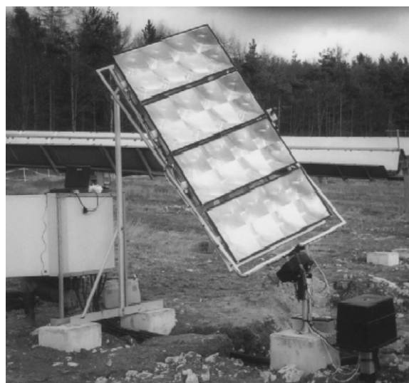
Fig. 3. Multiple point-focus Fresnel lenses, mounted in gimbals, with closed-loop tracking about both axes [33].
