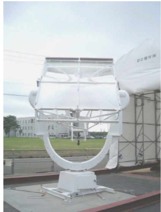
Fig. 11. Solar-pumped laser setup using Fresnel lenses [54].
