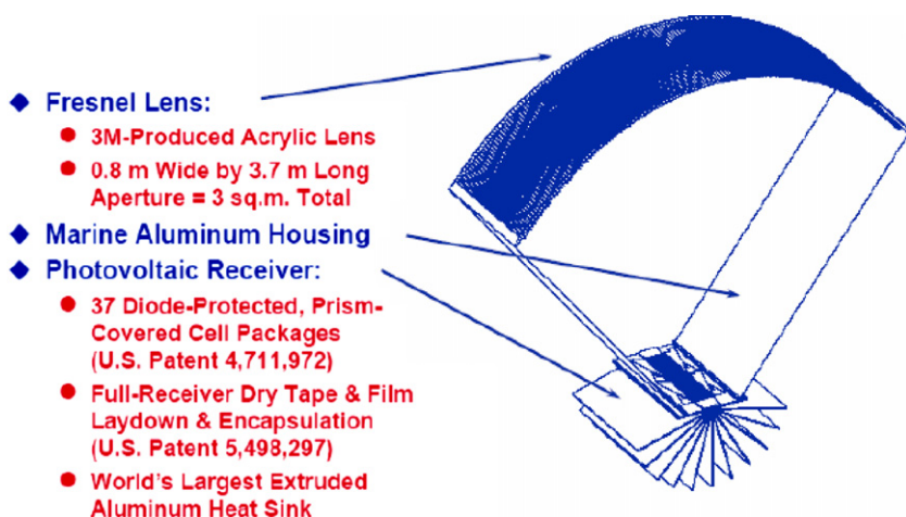
Fig. 13. ENTECH's fourth-generation concentrator module [63].
