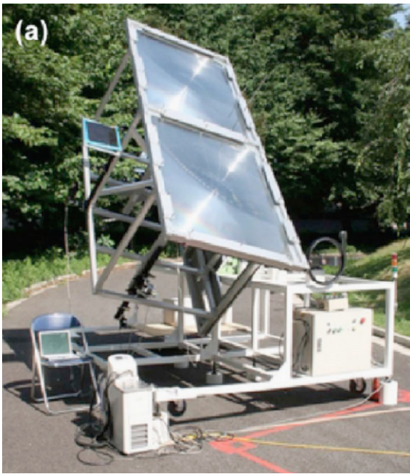
Fig. 10. Test system for laser from natural sunlight. Two pieces of Fresnel lens are used. All the system was in one unit and moves together. Once alignments of the laser cavity were fixed, realignment would not be necessary even if all the system moved following the sun [53].
