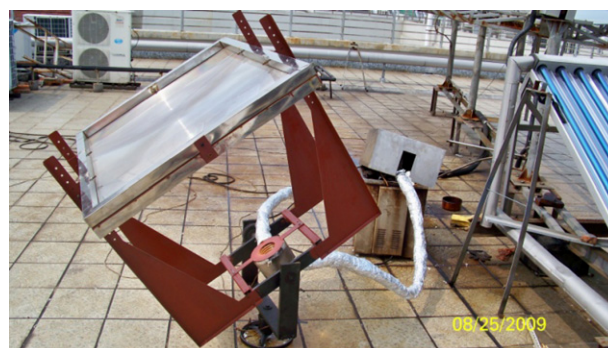
Fig. 23. The point-focus Fresnel lens solar collector and test system [106].
