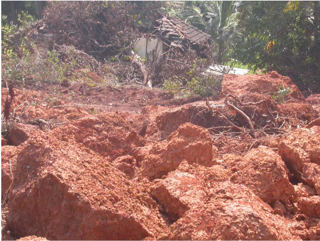
Fig.2.15: Soft laterite in the slide materials at Kadwad Landslide-2
