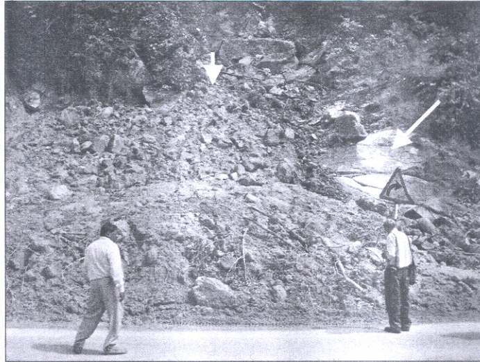
Photo15: View of the slide with exposed shallow dipping plane (right arrow) and mafic dyke boulders (left arrow)
