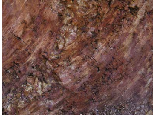
Fig: 4.2. Partially formed soft laterite in Zariwada landslide at Kadwad (lack of erosion due to water logging may be the cause of this formation)
