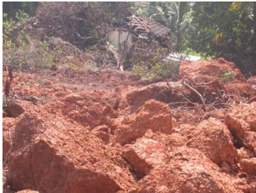
Fig: 4.3. Imperfectly evolved soft laterite in the Zariwada landslide at Kadwad
