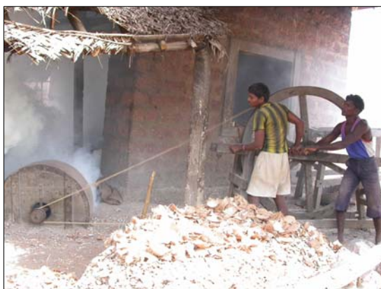
Figure 3.1: Bivalve shells burnt along with coconut shell to make lime powder.
