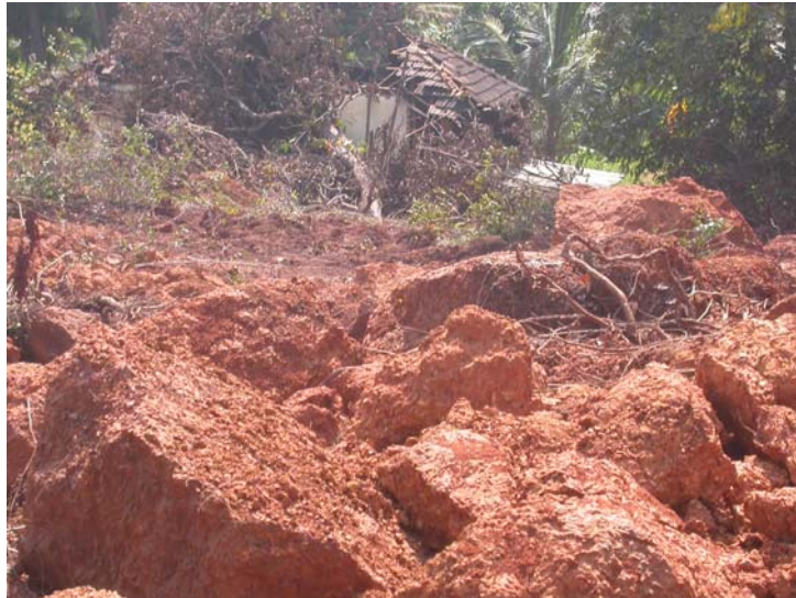
Figure 6: Incompletely formed laterite due to water logging in Kadwad-2 landslide
