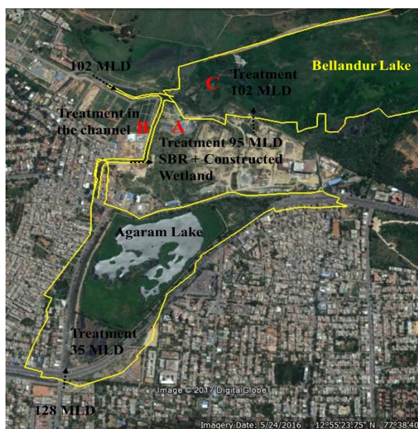
Figure 3.3.1: Proposed Sewage Treatment with wetlands
