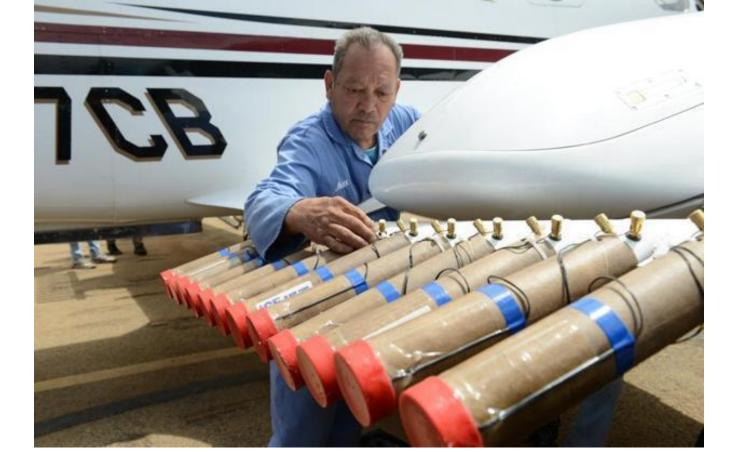
The Beechcraft King aircraft uses silver iodide, potassium chloride and sodium chloride—chemicals that can aid precipitation when seeded into rain-bearing clouds. Photo: Hemant Mishra/mint
