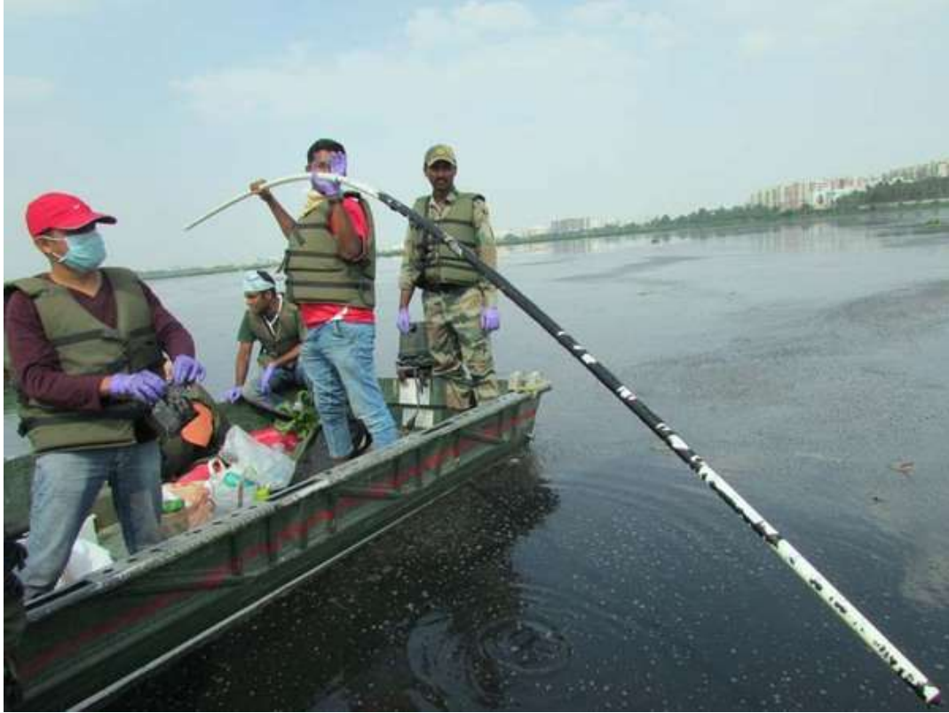
Bathymetric survey under progress at Bellandur lake. Researchers measure the sediment thickness and depth of the polluted lake. Pic: Akshatha M
