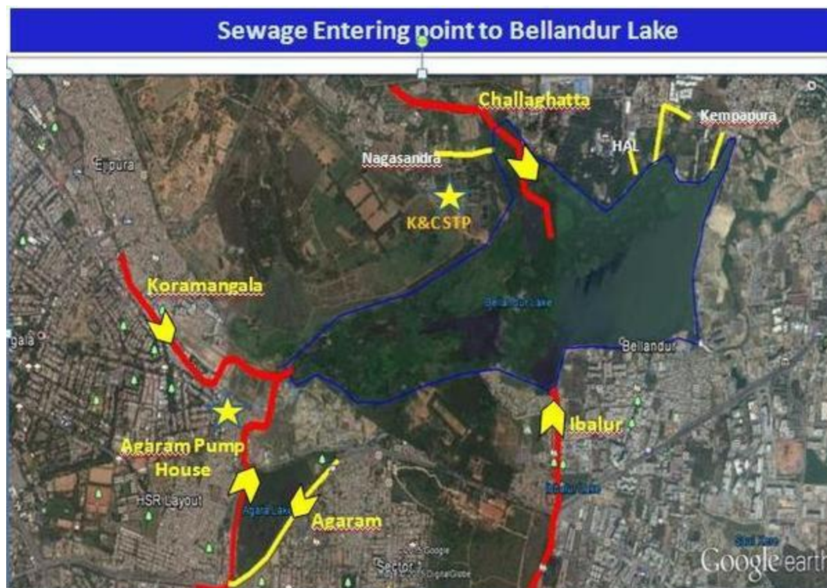
Graphic representation of four main inlets from where sewage enters Bellandur lake. Pic Source: BWSSB
