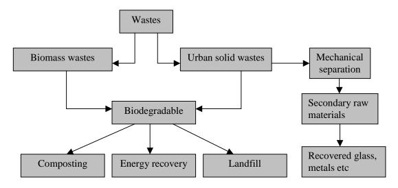
Fig 2.2. Pathways for solid waste treatment for recovery and recycling process.
