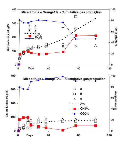
Fig 4.26. Cumulative gas production pattern of mixed fruits and orange mixture.
