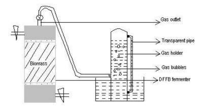
Fig 3.7. Sketch of DFFBR showing gas measured by downward displacement of water.
