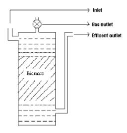
Fig 3.6. Sketch of laboratory scale DFFBR
