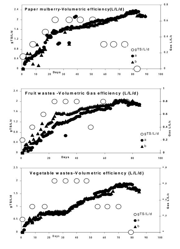
Fig 4.13.Volumetric efficiencies and gas production pattern of feedstocks in run 2 experiment
