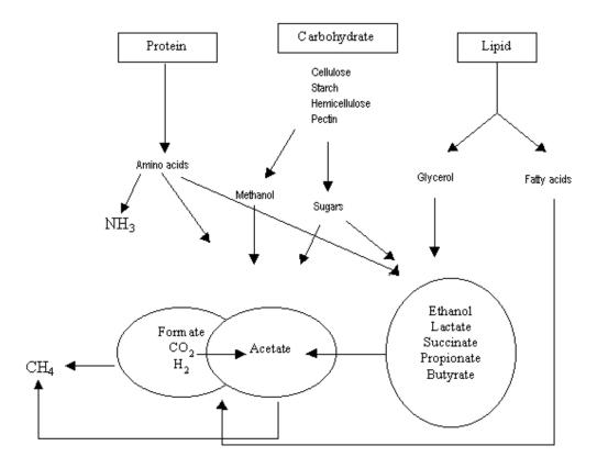
Fig 2.5. Anaerobic breakdown of complex organic matter.
