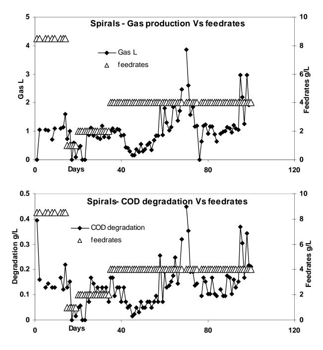
Fig 4.32. Feed rates Vs Gas production and COD degradation for spirals
