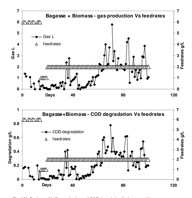
Fig 4.33. Feed rates Vs Gas production and COD degradation for bagasse + biomass
