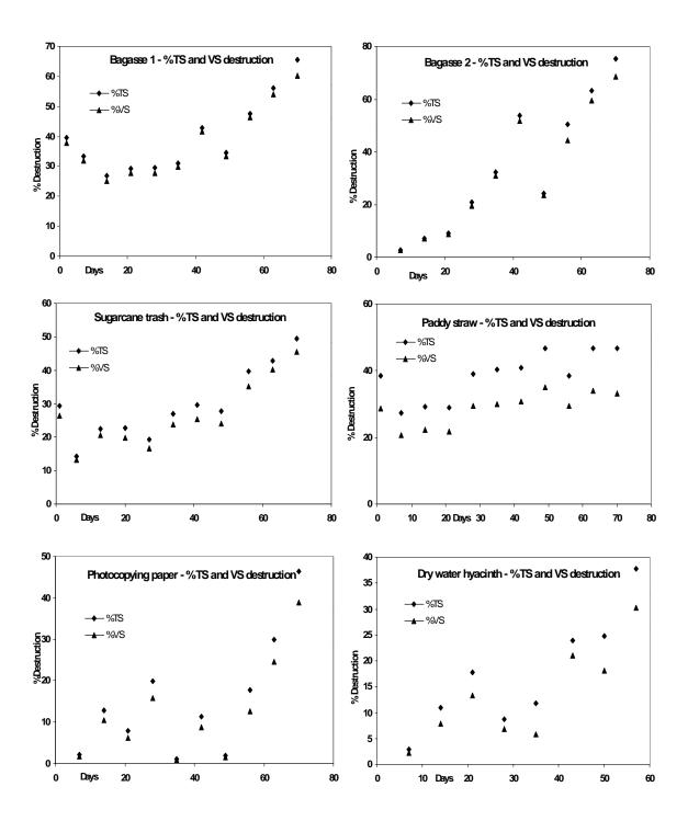
Fig 4.11. TS and VS destruction of dry feedstock.
