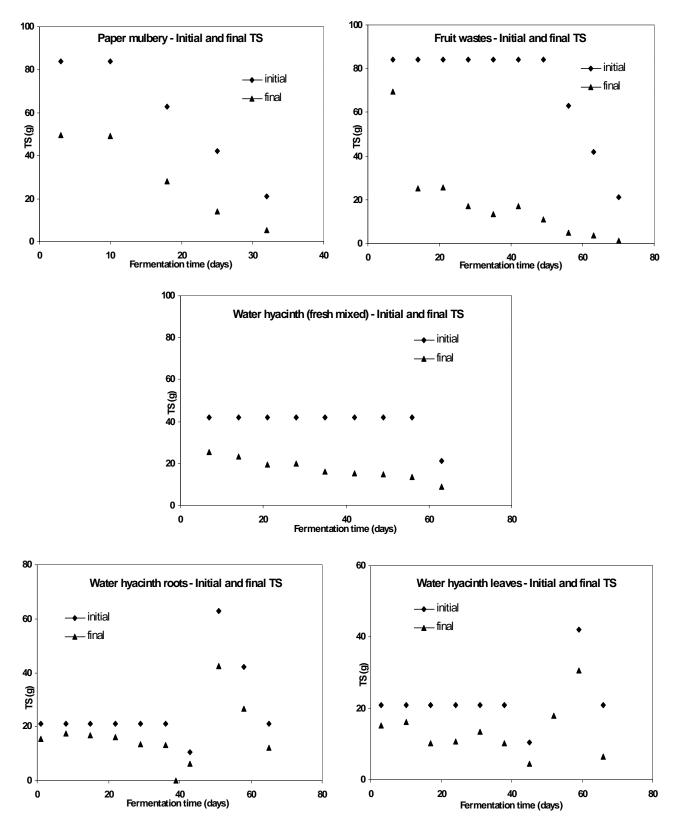
Fig 4.10. Changes in TS before and after fermentation in fresh feedstocks.
