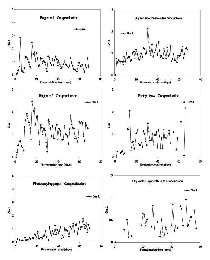
Fig 4.3. Daily biogas production rates from dry feedstocks.
