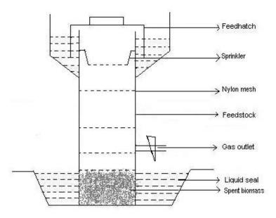
Fig 3.1. Sketch of SSB reactor.
