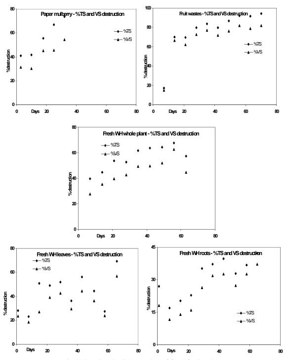
Fig 4.12. TS and VS destruction of fresh feedstock.
