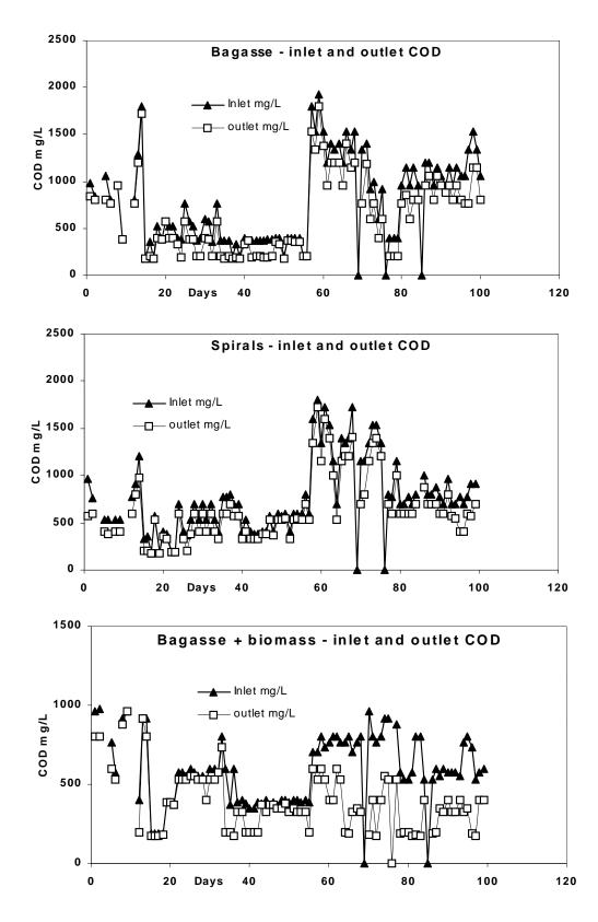
Fig 4.34. COD reduction in DFFBR reactor.
