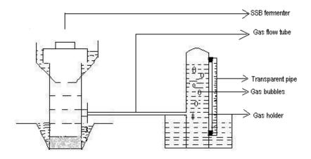
Fig 3.2. Sketch showing gas measurement by downward displacement of water.
