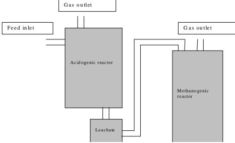
Fig 2.7.Two-step digestion
