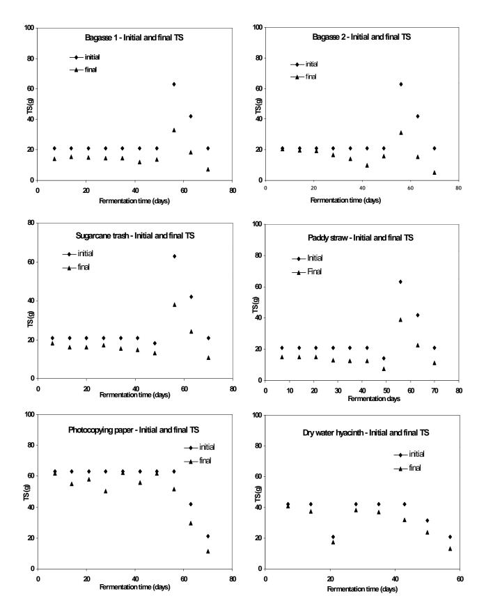
Fig 4.9. Changes in TS before and after fermentation in dry feedstocks.
