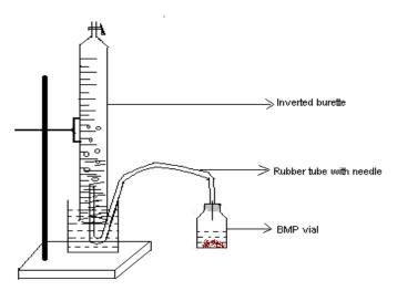
Fig 3.5. Sketch showing the set-up used for measurement of gas production from BMP vials
