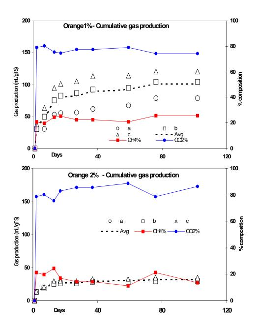
Fig 4.23. Cumulative gas production pattern of orange peel.
