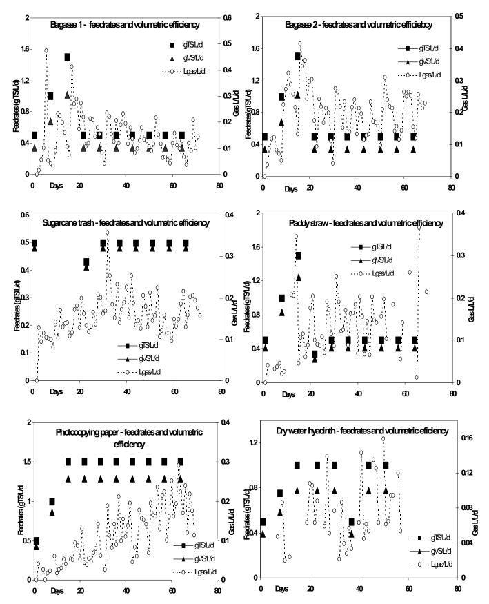
Fig 4.5. Feed rate Vs volumetric efficiency in dry feedstock
