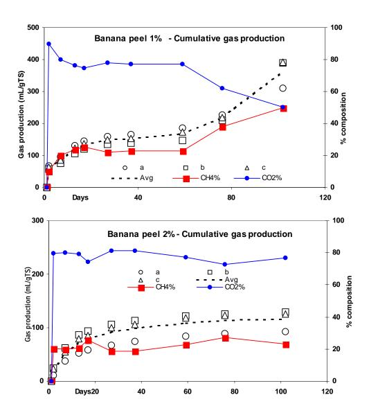
Fig 4.21. Cumulative gas production pattern of banana peel.
